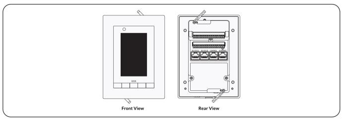
**2** The KX4 Touchscreen has the following built-in components: ambient and proximity sensors and reset button.
