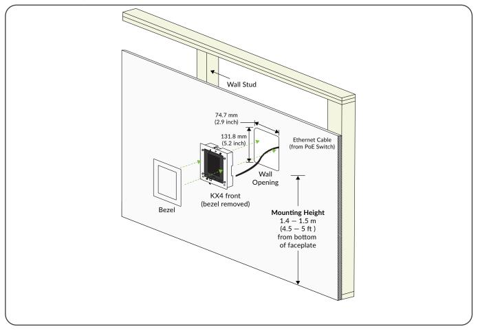
**Note:** There is little margin for error when fitting the KX4 Touchscreen into the wall opening. Make sure to use the included cardboard cut-out template to create the correct size opening in the wall. Additionally, carefully double-check that all measurements taken using the cardboard cut-out template are accurate.
