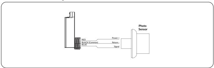
**3** SIM to Sensor Junction Box Wiring
