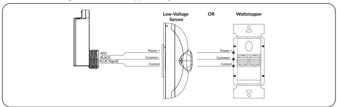
SIM to Photo Sensor Wiring
