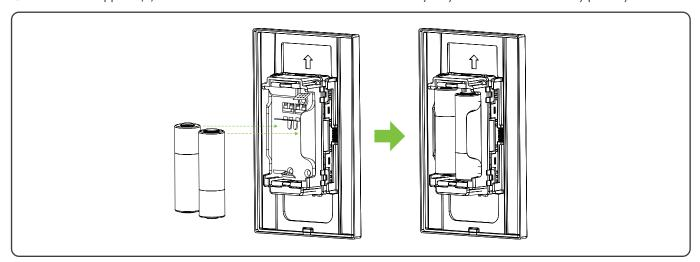
3 Place the Wireless Wallstation assembly into the mounting plate and push gently until 'clicks' are heard. This confirms that the pieces are secured.
