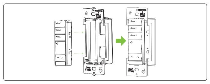
Install the mounting bracket using the supplied screws. Install the "Decora" sytle wall plate using screws supplied with the wall plate.
