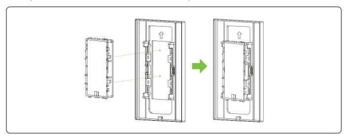
**5** Attach the Wireless Wallstation assembly to the surface mount kit until it snaps in.
