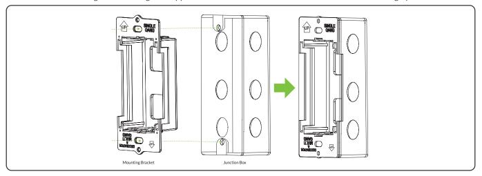
Option 2 — Low-Voltage Device Box Installation Install the mounting bracket using the supplied screws. Ensure that the MULTI GANG label is facing up.
