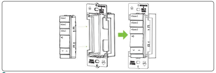
Install the mounting bracket using the supplied screws. Install the "Decora" sytle wall plate using screws supplied with the wall plate.
