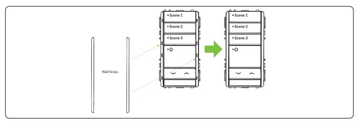
Orient the mounting bracket such that the DECORATOR and MULTI GANG labels are facing up. Insert the wallstation button assembly into the mounting plate until 'clicks' are heard. Clicks confirm that the pieces are secured.
