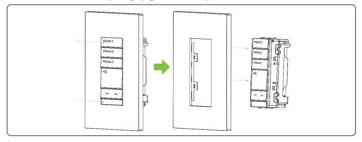
2 Install the supplied wall strips to the button assembly until they snap in.
