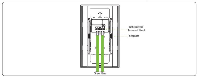
Notes: GreenBus wires should not be crossed and are polarity independent. A short GreenBus jumper can be used to interconnect ganged wallstations. GreenBus wires can be inserted into either of the 2-ports. Press the corresponding button to insert the wires.
