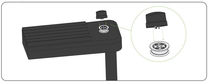
2 Mount the control with the arrow and 'N' on the cover facing north.
