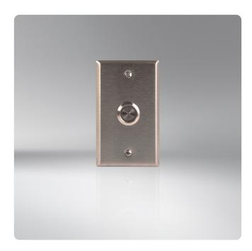
The INDPB (Industrial Push Button Wallstation) is a single-zone, wall-mounted user interface that provides local on/off control over a lighting zone. Utilizing a standard single-gang junction box form factor in a rugged stainless steel housing, it connects to the Encelium X Lighting Control System through a GreenBus cable with standard 2-pin connectors.
