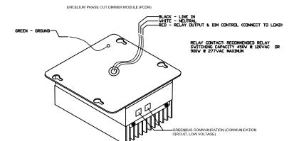
ENCELIUM PHASE CUT DIMMING MODULE (PCDM) - WIRE TABLE
