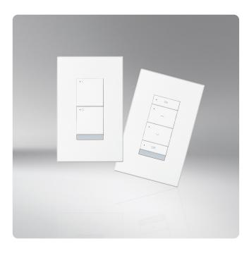
The WS Standard Wallstation series consists of a two-button and a four-button wallstation that enable essential lighting control. The 2-button wallstation is a single zone manual controller ideal for conference rooms, private office, classrooms and other similar spaces. A short press of the upper/lower buttons turns lighting ON/OFF, while a "press and hold" dim lighting up or down.
