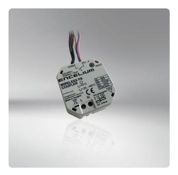
The Encelium **Wireless Push Button Coupler (WPBC)** enables convenient control of light levels and allows use of any standard push button or switch as an input device to the Encelium X Lighting Control System. The WPBC gives you the flexibility to select the brand, shape, color and size push button or switch preferred for your lighting design. Simply install the WPBC in any standard flush-mount junction box, connect it to mains power, and your selected wall switch.
