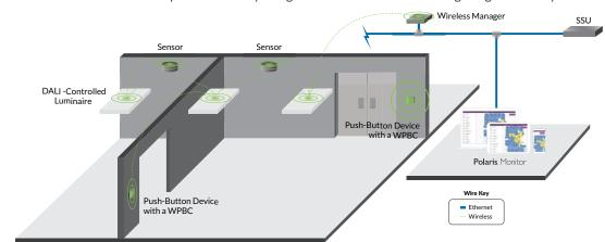
This illustration shows how each component is easily integrated into the Encelium X Lighting Control System.
