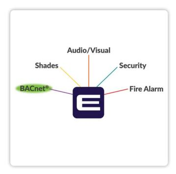
The Encelium **BACnet®** Interface enables the integration with any BACnet compatible building automation system. The BACnet interface resides in the Encelium SSU and operates autonomously providing access to lighting and sensor statuses as well as control via BACnet. The connection between the two systems is established via BACnet/IP.
