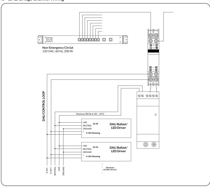
**2** Class 1 Wiring — DALI Bus can be run as Class 1 (Consult applicable electrical and building codes).
