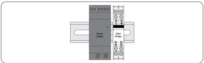
Do not reverse the 24 VDC polarity connections from the power supply to the DALI Bridge or damage may result.
