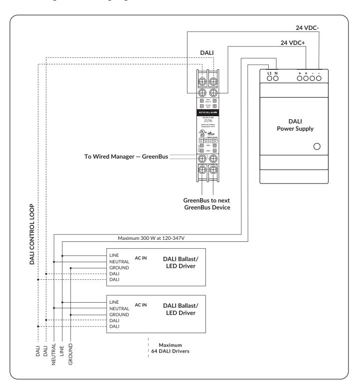
**2** DALI Bridge Wiring Diagram
