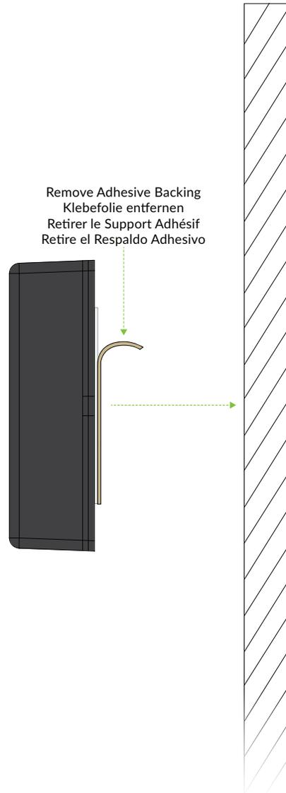
Attach the adhesive to the back of the device by removing adhesive backing from both adhesives and press device on the flat, clean surface with pressure for 30 seconds.
