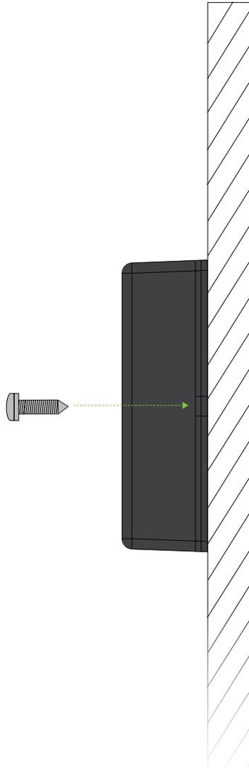
The Dry Contact Input Interface may be screwed directly to a wall surface.
