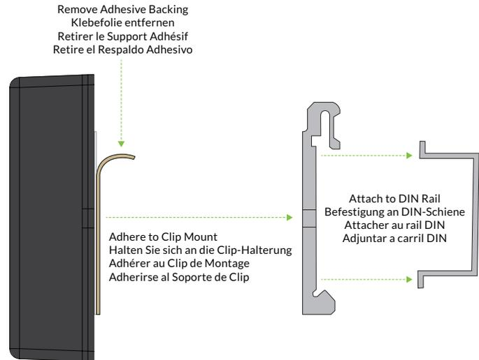
Remove one liner from both adhesive strips and press on to the DIN rail clip for 30 seconds. Then mount the DIN rail clip to the DIN rail.
