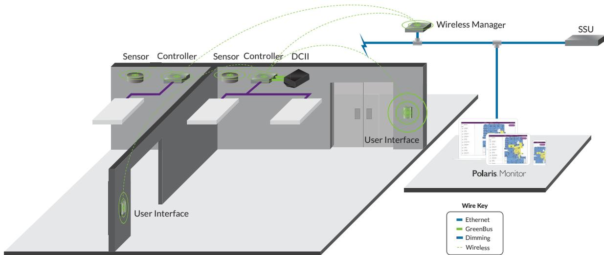
In a wireless system, the DCII is tethered from the GreenBus ports on the load controllers (WCM or WALC).
