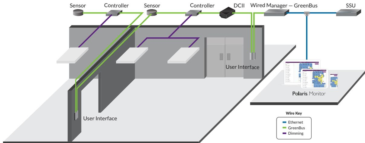
The DCII is a GreenBus device and is wired using the 2-wire input/output cables in a daisy chain wiring scheme. It can be located in a ceiling or in AV closets depending on the application.
