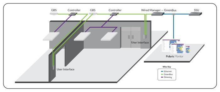
Note: As the modules obtain power via the GreenBus, the number of modules on each chain is limited. Encelium suggests leaving room for future system upgrades and limiting the number of modules per chain to 100 units during initial installation.
