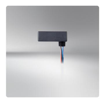
The Wireless Control Module (WCM) is a key component of the Encelium system. Individually addressable, the WCM enables each ballast or LED driver to be independently controlled and configured to meet the facility's needs. The WCM switches a fixture ON or OFF via a relay contained in the module as well as delivers a low voltage dimming signal to any 0-10V dimming ballast/LED driver.
