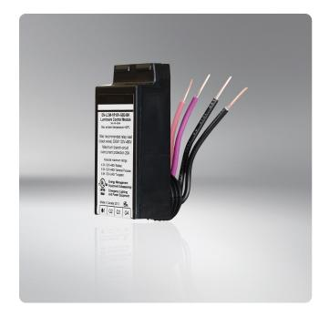
The Wired Luminaire Control Module (LCM) is a 0-10V luminaire level load controller with an internal relay capable of switching AC loads. Similar to other GreenBus devices, the LCM receives power and communication from the Wired Manager. The device is configured to meet the lighting control strategies using Encelium X.
