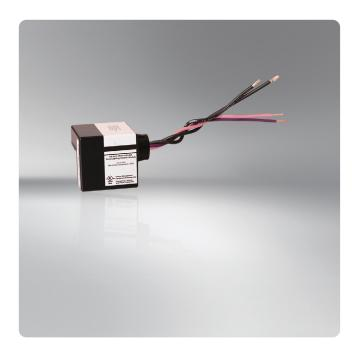
The Area Lighting Controller (ALC) provides a high-power switching and dimming interface between a group of luminaires and the GreenBus™ communication network. Individually addressable with the Encelium X Lighting Control System, the ALC switches a single wired zone of multiple luminaires ON or OFF via an integral high current relay while setting the zone's overall light level with a 0-10V dimming output wired to the luminaires' dimming ballasts or LED drivers.
